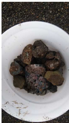
Foto 2: S2 slakken fundatie (boringen 103, 104 en 105)
