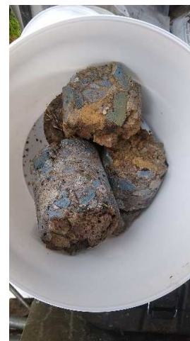
Foto 3: S3 slakken fundatie (boringen 106, 107 en 108)
